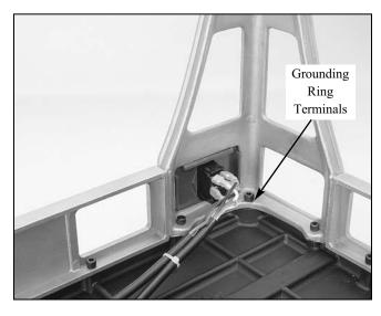
Figure 10. Attaching the grounding ring terminals.
